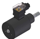
Example 6: ECH75-20E Modification of ECH75-20, the shaft has been plucked, from \varnothing 12 to \varnothing 14 , and one of the thread has been removed
