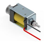
Protection rate: IP00 Insulation class: Y (90°C) Reference cycle: 3 minutes Standard stroke (s): 8 mm Temperature rise "ΔV31": 70°C Working temperature: -10 to 45°C Work: Push / Pull
