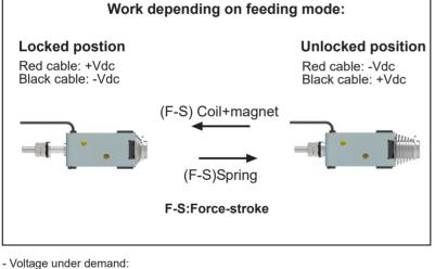
They can be manufactured at voltages between the maximum and minimum voltage values shown in the chart.
