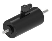
Protection rate: **IP40** Insulation class: **B (130°C)** Reference cycle: **5 minutes** Standard stroke (s): **25 mm** Temperature rise " $\Delta$ V<sub>31</sub>": **70°C** Working temperature: **-10 to 45°C** Work: **Push / Pull**
