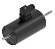
Protection rate: **IP40** Insulation class: **B** (130°C) Reference cycle: **5 minutes** Standard stroke (s): **30 mm** Temperature rise " $\Delta V_{31}$ ": **70°C** Working temperature: **-10 to 45°C** Work: **Push / Pull**
