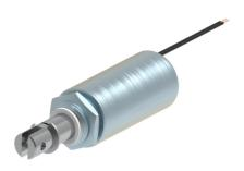
Protection rate: IP30 Insulation class: B (130°C) Reference cycle: 2 minutés Standard stroke (s): 12 mm Temperature rise "∆V31": 70°C Working temperature: -10 to 45°C
