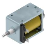
Protection rate: IP00 Insulation class: B (130°C) Reference cycle: 5 minutés Standard stroke (s): 10 mm Temperature rise " $\Delta V_{31}$ ": 70°C Working temperature: -10 to 45°C Work: **Push** / Pull
